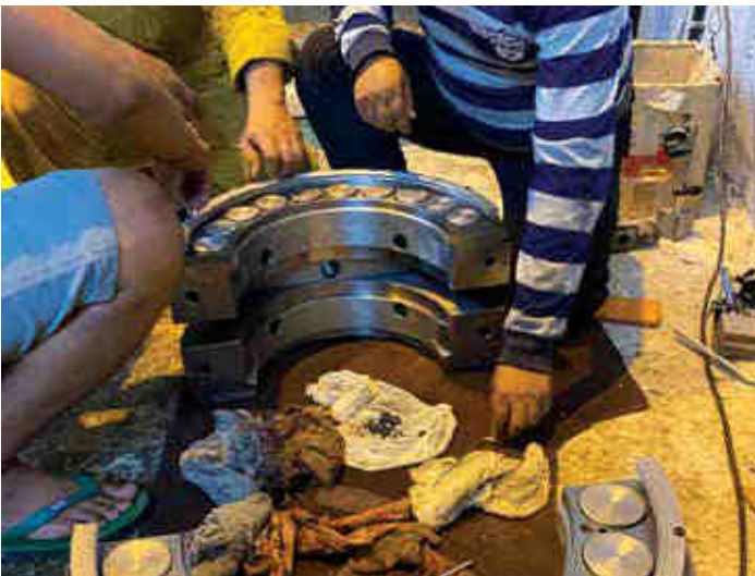
▶ Maintenance of Bearing
